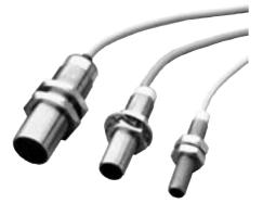
The D Series comes in three sizes, all in the easy flush mount type. Both NPN (sinking) or PNP (sourcing) types are available. They sense any conductive metal surface within range of their sensing coils. They do not require a magnetic target and are perfect for our ratemeters and counters. An LED indicator lights during activation.
